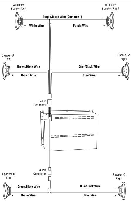
This unit for use only with a 12 Volt DC power source with a negative ground.
